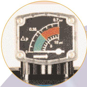
The direct mounting differential pressure gauge is calibrated for accurate running cost measurement and has a remote sensing option. Fitted as standard on filters 3/4" and larger (except Grade D & CD filters).
